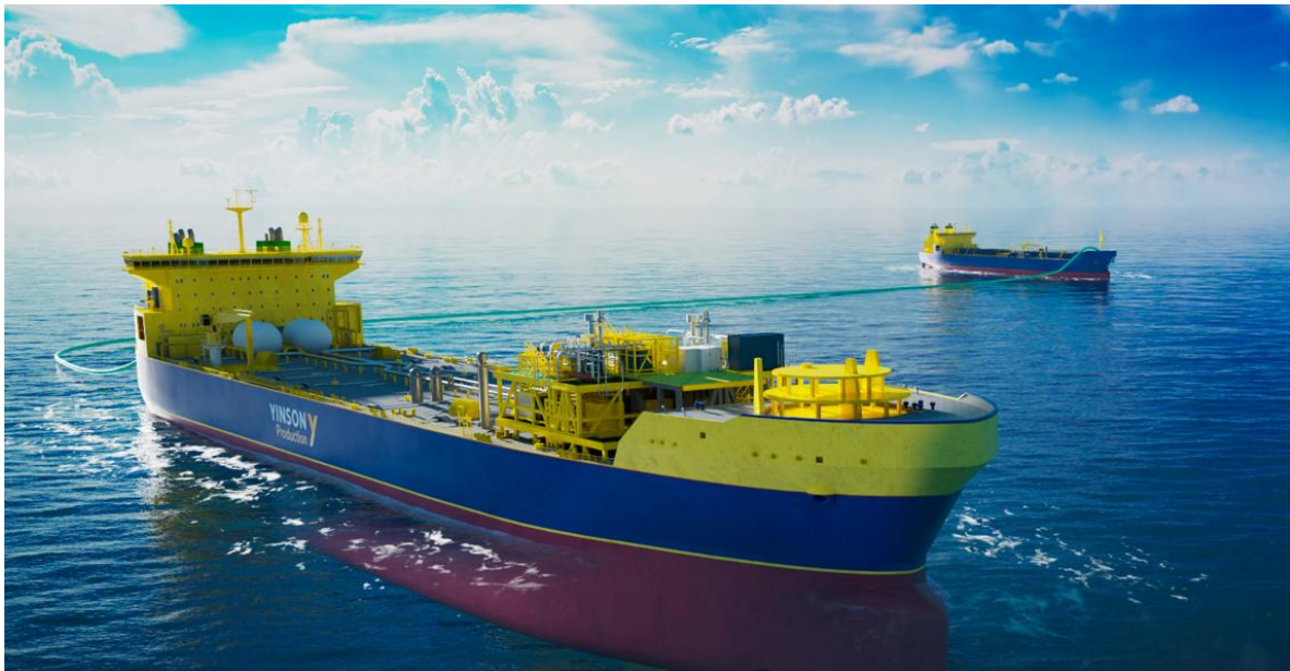
An illustration of a FSU in the foreground, receiving cargo from a LCO2 carrier in the background.
